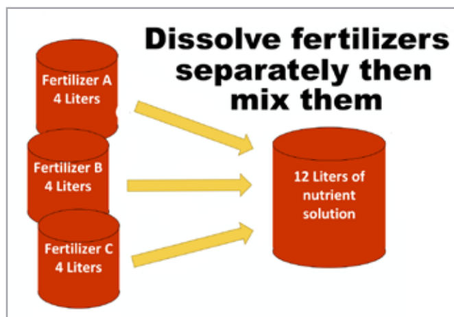
Figure 2. Hand mixing fertilizers: dissolve each fertilizer formulation in separate containers, they can be combined once dissolved.
