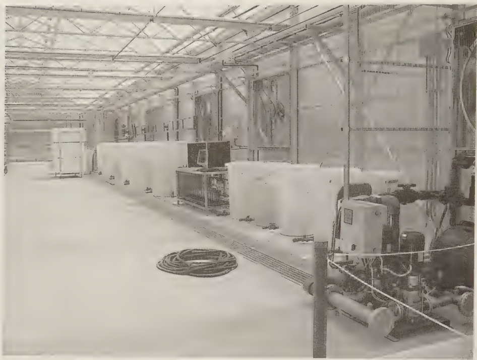
FIGURE 5.34 Adjustment of the nutrient solution using an injection system. (From Hydronov, Inc., Japan Plantation Co. Ltd.-Nippon-Noen, Hiroshima, Japan. With permission.)
