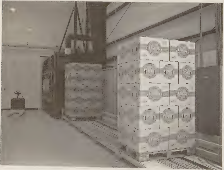
FIGURE 5.32 Boxed lettuce moving through a vacuum cooler. (From Hydronov, Inc., Hydroserre Mirabel Inc., Tennessee, Livingston, TN. With permission.)
