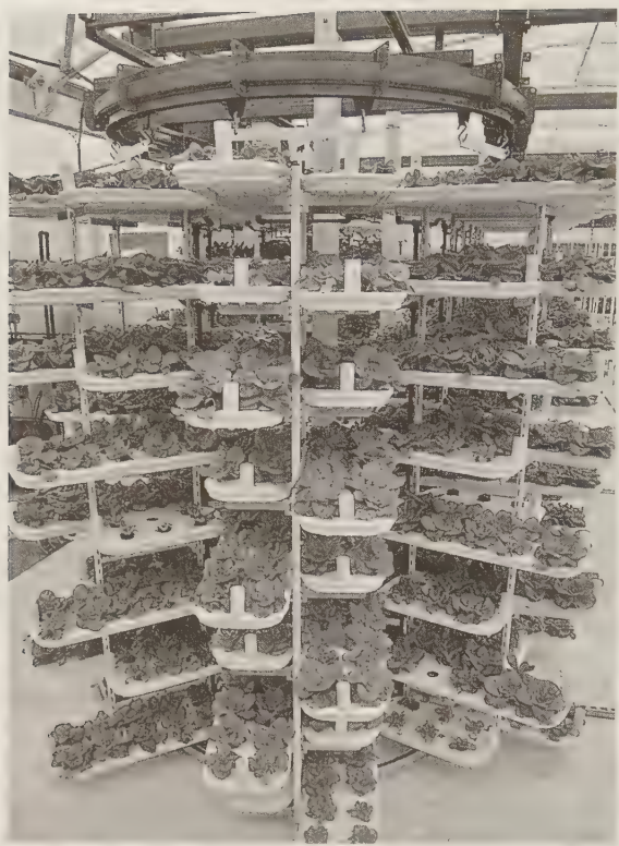
FIGURE 13.46 VertiCrop system where overhead conveyor curves back to change direction. (From Valcent Products [EU] Ltd., Cornwall, UK. With permission.)
