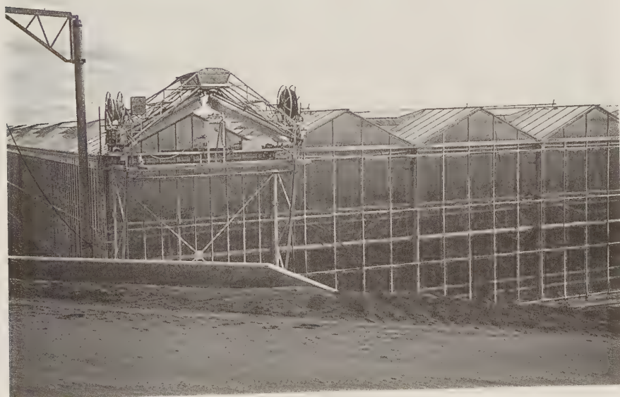
FIGURE 10.52 Machine to whitewash and wash the greenhouse roofs. (From Eurofresh Farms, Wilcox, AZ. With permission.)
