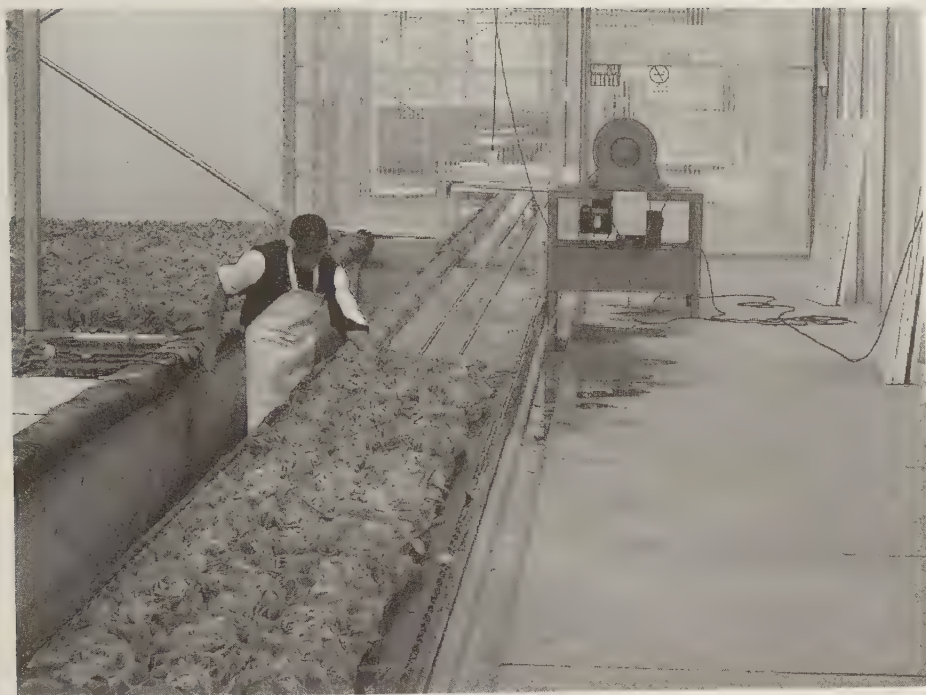
FIGURE 5.29 Lettuce traveling on conveyor system to packing facility. Note: The winch that pulls the boards to the harvesting end of the lettuce raft pond. (From Hydronov, Inc., Omnilife Hydroponic Greenhouses, Leon, Mexico. With permission.)
