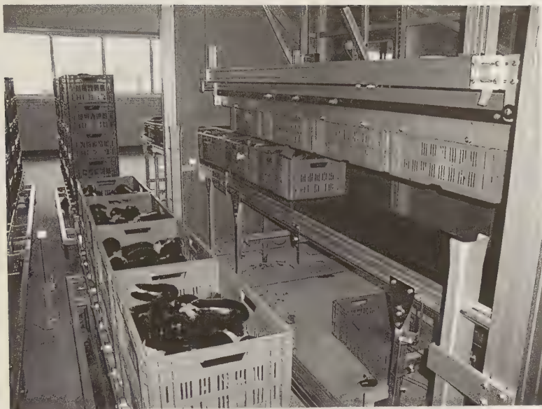
FIGURE 10.48 Eggplants in tote bins are automatically unloaded. (From FormFlex/Metazet Zwethove B.V., The Netherlands. With permission.)
