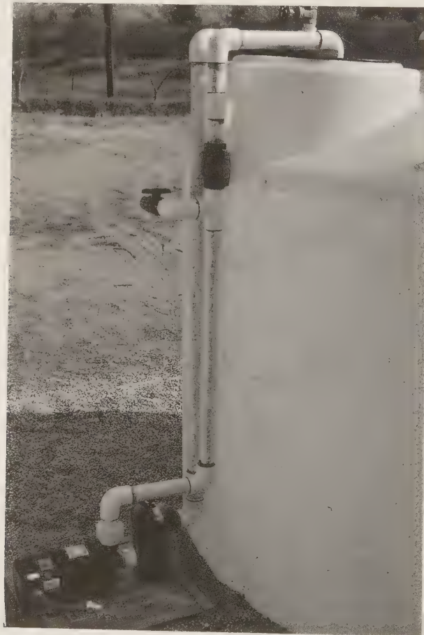
FIGURE 3.8 Circulation pump with plumbing to agitate the stock solution. (From California Watercress, Inc., Fillmore, CA. With permission.)
