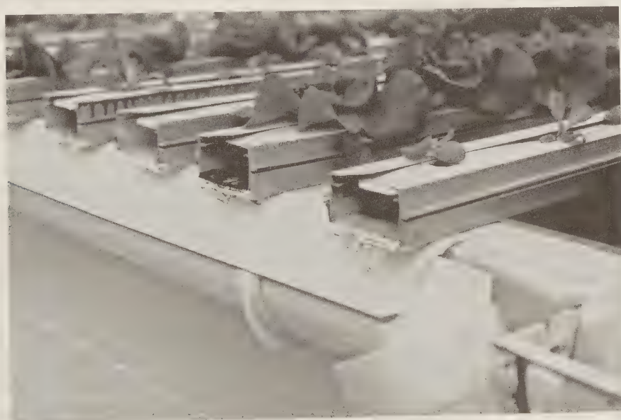
FIGURE 6.20 Aluminum NFT channels exit to a catchment pipe that returns nutrient solution to a cistern. (From F.W. Armstrong Ranch, Oak View, CA. With permission.)
