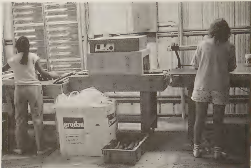
FIGURE 10.19 Cucumbers may be shrink wrapped with an L-bar sealer. (From Environmental Farms, Dundee, FL. With permission.)
