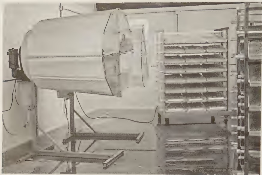
FIGURE 5.49 Alfalfa sprout growing systems of racks and rotary drums.
