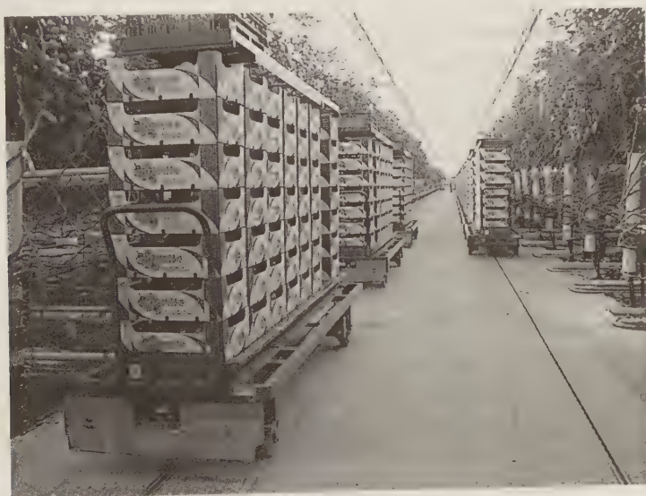
FIGURE 10.45 Carts moving in the central passageway on the chain track system. (From FormFlex/Metazet Zwethove B.V., The Netherlands. With permission.)
