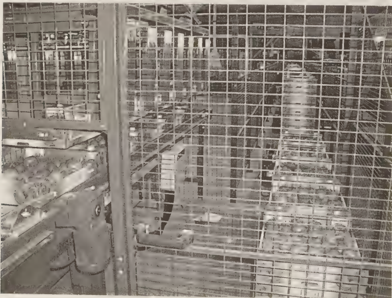
FIGURE 10.36 Machine lifts boxes from picking carts and places them on the grading–packing belt. (From Eurofresh Farms, Wilcox, AZ. With permission.)
