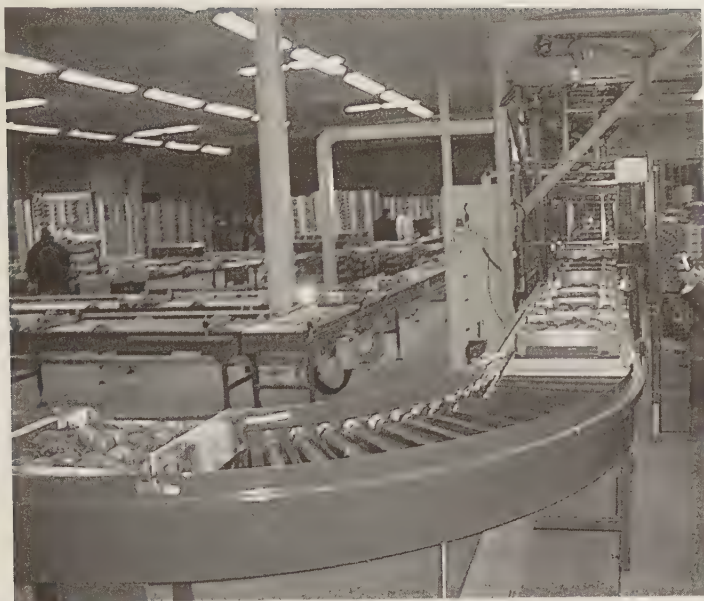
FIGURE 10.37 The machine lifts the cases of tomatoes from the picking carts. (From Eurofresh Farms, Wilcox, AZ. With permission.)
